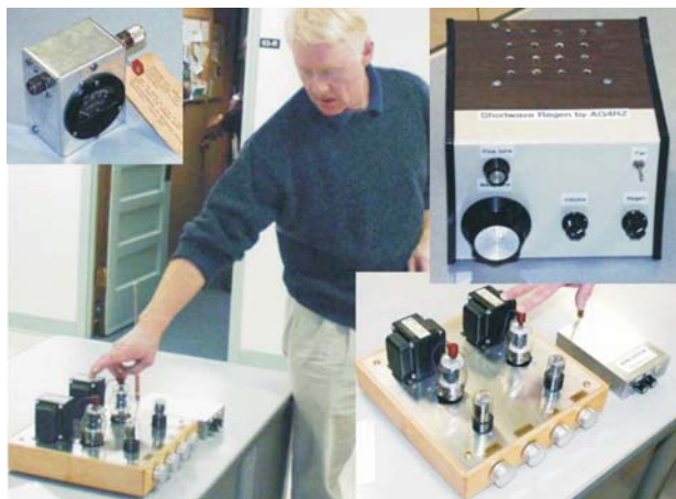
Clockwise from upper left: W4DCW's carrier-null meter made from aluminum rescued from old transcription disk. James H4HCJ's winning tube amplifier; a very nice regenerative receiver from Tim, AG4RZ; lower right, James' tube amp & 6-meter transceiver.
